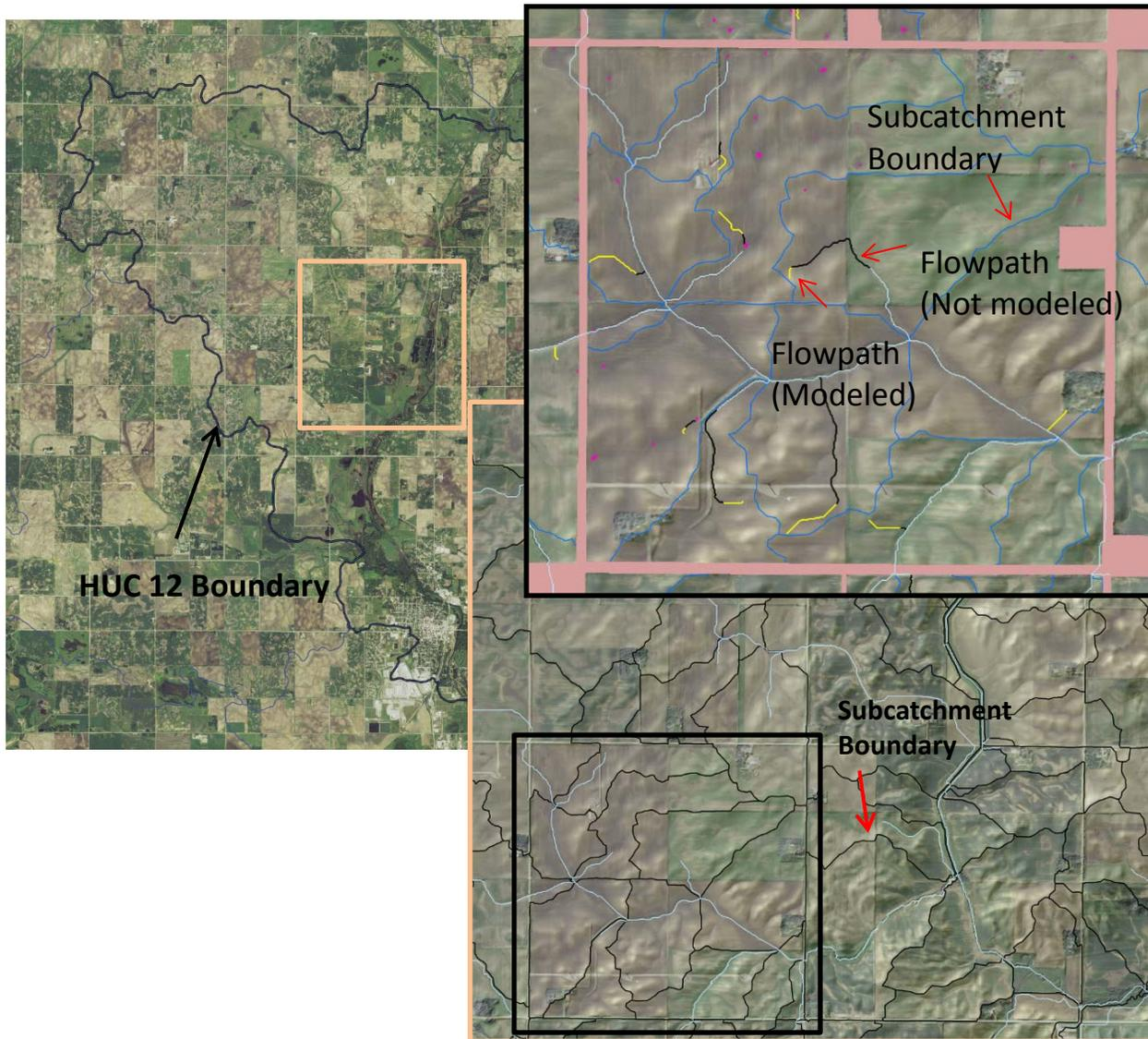
Figure 1. Diagram of HUC 12 Boundary (left), Subcatchment Boundary (lower right inset), and Modeled and Non-modeled Flowpath Elements (upper right inset)
