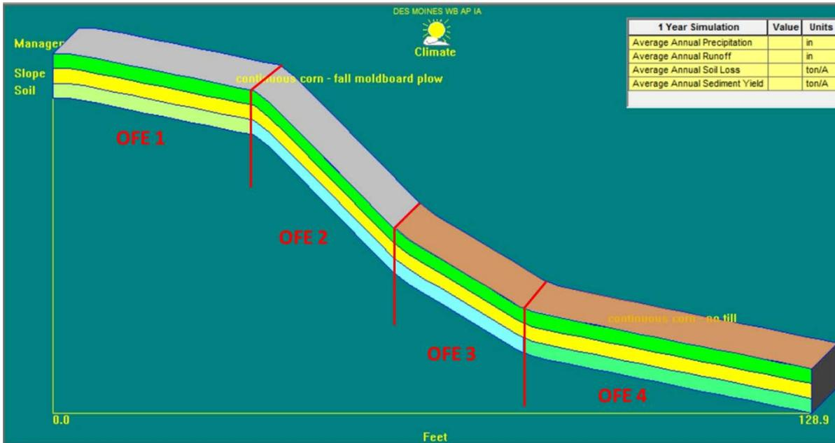
Figure 2 Example WEPP Overland Flow Element (OFE) diagram showing three unique soils and two unique managements.
