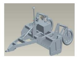
Fig. 1 Mechanical structure of GNSS land leveling equipment
