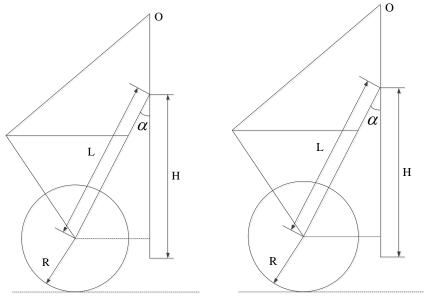
(a) the cylinder is extended (b) the cylinder is shortened
