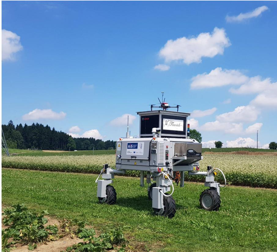
Fig. 2. Unmanned Ground Vehicle Bonirob, carrying an Unmanned Aerial Vehicle.
