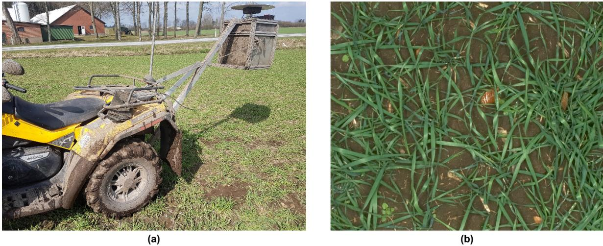
Fig. 2 (a) Camera platform attached on the back of an ATV, (b) Sample image acquired at about 40km/h
