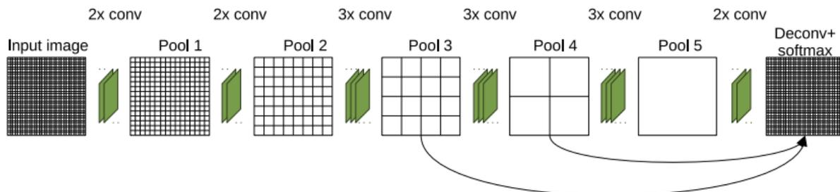
Fig 3. Overall overview of the utilized FCN model (Skovsen et al. 2017)
