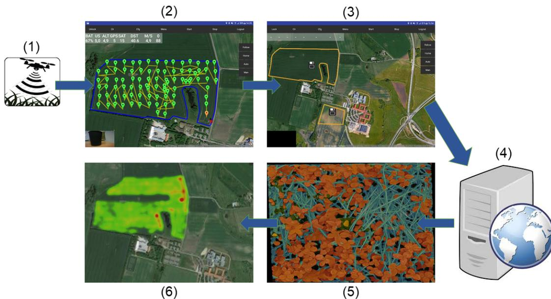
**Fig 10. Dataflow of utilizing the presented model together with a commercially available UAV. The flight plan and context are controlled by an Android application and the analysis is done via cloud computing. The result is a grass-clover ratio map, which can be utilized for management of fertilization**
