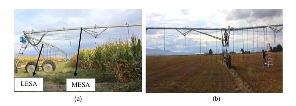
Fig. 1. LESA and MESA installed in the study area (a) Corn field (b) spearmint field. The emitters of LESA, as seen, are closer to the ground than MESA. Also, the outlet spacing of emitters in LESA is less by 3-6 m (10-20 ft).
