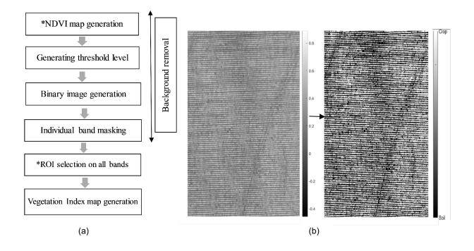
Fig 4. (a) Flowchart for data processing (\*ROI-Region of Interest, NDVI-Normalized Difference Vegetation Index) (b) NDVI map of corn field before and after background removal and masking (Image of 49 Days after Plantation i.e. DAP).
