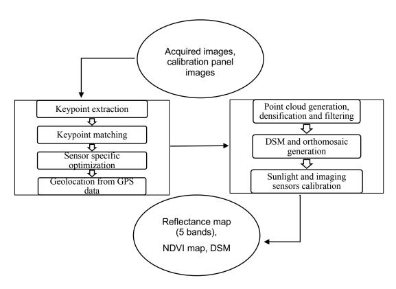
Fig 3. Image preprocessing workflow for multispectral images in Pix4D.
