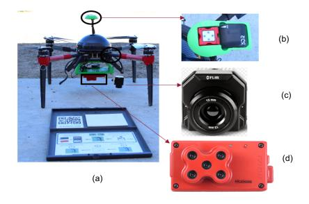
Fig. 2. The Data collection system (a) small UAS (b) a GPS receiver and downwelling light sensor (c) thermal infrared imaging sensor (d) multispectral imaging sensor.
