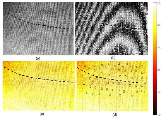
Fig. 5. Workflow of thermal imagery processing, 49 DAP corn field (a) selected thermal frame (b) frame after masking, with crop as black pixels and the soil background in white (c) colored frame, soil shown in white, red to yellow the temperature increases (15 to 40°C) (d) ROI selection, 30 from LESA and 30 from MESA. The scales are in °C. The white color represents soil in the colored frames.
