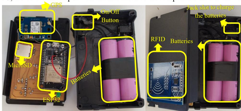
Figure 3: Electronic tracking device viewed internally, with the arrangement of the components used.
