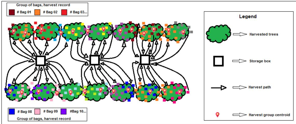
Figure 4: Scheme for estimating productivity considering method #1
