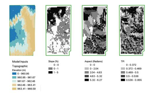
Figure 1A) 32 hectare Field A showing topographic input variables for modeling including panel 1) elevation, panel 2) slope, panel 3) aspect, and panel 4) topographic position index (TPI).
