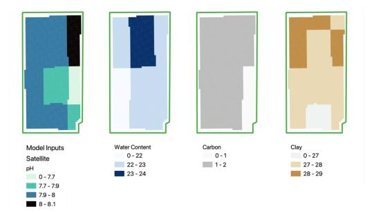
Figure 1B) 32 hectare Field A showing satellite input variables for modeling including panel 1) pH, panel 2) water content, panel 3) carbon content (%), and panel 4) clay content (%).
