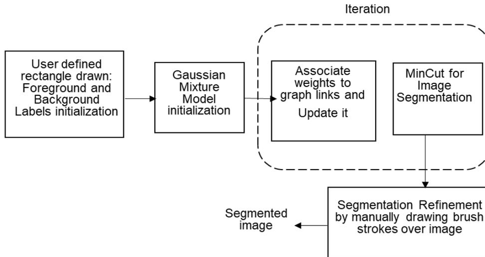
**Figure 2. A workflow diagram for image segmentation based on GrabCut algorithm.**
