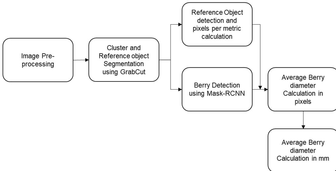
**Figure 5. Flow Diagram showing calculation of Average diameter of berries.**
