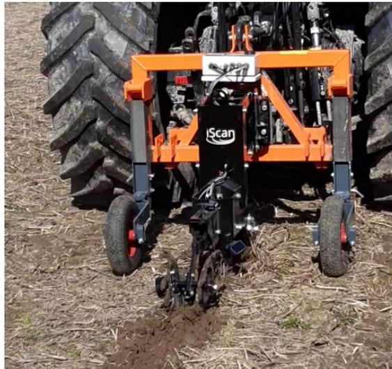
Fig 1. Veris iScan+ device, custom sub-frame for mounting the device and supporting wheels.
